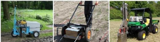
The Lightning is most commonly deployed on an electric wheeled or tracked vehicle to allow access over uneven slippery terrain.
