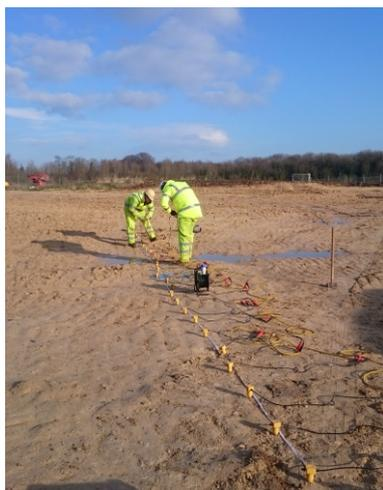
**B** A seismic survey set-up
