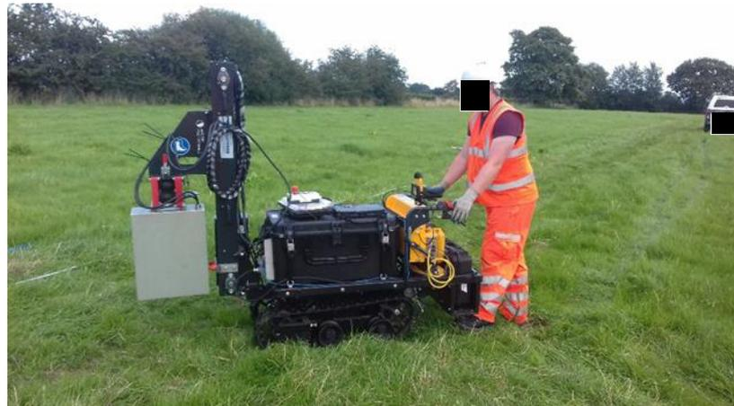
**Plate 4:** Seismic reflection data collection on site using the Mechatronics Lightning seismic source.
